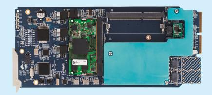
The MCD-1080 serves as a multichannel audio decoder specifically crafted for operations within FM/AM transmitter stations and monitoring environments.
