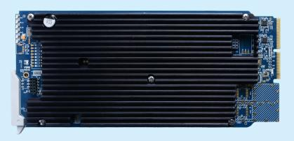
The DLY-3420 is a compact solution to apply desired delay on video, embedded audio, and four AES inputs. The uncompressed signals are directly delayed so that quality completely stays intact.
