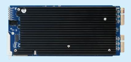
The CHO-3360 is an automatic/manual changeover module compatible with SRM frames. It accepts three 3G/HD/SD-SDI inputs and provides two independent groups of outputs. The clean and quiet switching can be triggered manually through GPIs and UI, or automatically based on the defined rules and priorities.
