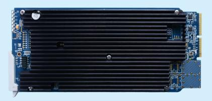
The UDC-3455 is a broadcast quality modular up/down/cross converter that can convert video format between 3G, HD, and SD. Frame synchronization (with video timing adjustments), color correction, image enhancement, and aspect ratio conversion (with AFD support) are supported in the video processing path.
