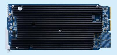
The SAE-3390 is a compelling and flexible solution for embedding eight audio pairs to a 3G/HD/SD-SDI signal from analog/digital audio inputs or previously embedded audio channels. The audio processor core can delay audio pairs for up to 10 seconds and apply desired gain. The module also features optical I/O, frame synchronization, timing adjustment, ancillary data transparency, and test tone/pattern generation.
