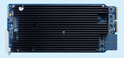
The SAD-3395 is a highly flexible solution for de-embedding eight audio pairs from a 3G/HD/SD-SDI signal and routing them to analog/digital audio outputs. The audio processor core can delay audio pairs for up to 10 seconds and apply desired gain. The user can also embed processed and shuffled audio back to the SDI signal.
