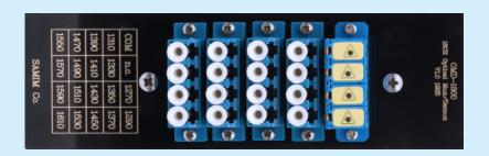
The OMD-1800, as a CWDM optical mux and demux, is a bidirectional passive optical multiplexer and de-multiplexer, allowing multiple optical signals at different wavelengths to pass through a single optical fiber link.
