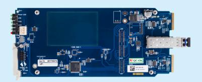
The OED-3904 is a converter of optical digital video signals to 3G/HD/SD-SDI or DVB-ASI electrical signals. The module can receive two video signals over fiber optic links via an SFP and provide four electrical outputs per channel.
