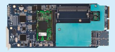
The IIP-2000-CSIR is a complementary component of the Samim Intercom System, designed to seamlessly integrate eight channels of analog audio input and output (line-level) into the intercom system via a network connection. This product facilitates the establishment of audio connections between intercom panels and the CCU of studio cameras, audio mixers, microphones, or speakers.
