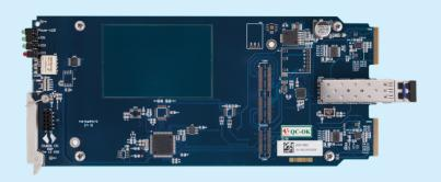
The EOD-3902 is a 3G/HD/SD-SDI/ASI electrical signals to optical signals converter. The module can transmit two digital video signals over fiber optic links and additionally provide two re-clocked electrical outputs per input.
