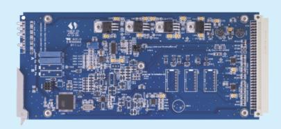
The AVD-0318 is an analog video distribution amplifier with cable equalization and eight outputs. This module provides single-ended input with passive loop-through.
